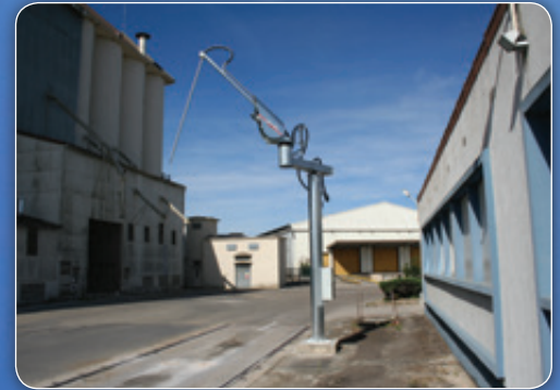
HERON Gyroscopic style offers operating ranges with 3300mm, 4100 mm, or 5000 mm radius.
